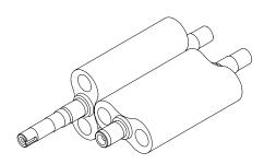
The RD pumps are positive displacement roots vacuum pumps. The pump bearings, gears and seals are lubricated by oil fed from oil reservoirs at either ends of the roots pump. A series of seals stops the oil from reaching the vacuum side of the pump. Roots pumps helps in shifting the operating pressure to a high vacuum range due to rotation of gear timed rotors in opposite directions. Roots vacuum pumps are capable of improving the attainable ultimate pressure of a pump system by a factor of 10.
